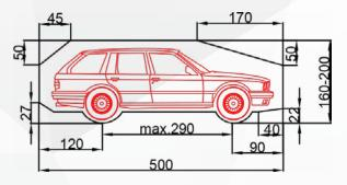
The total car height includes roof rail and antenna. Car height must not exceed the above max.car dimensions
