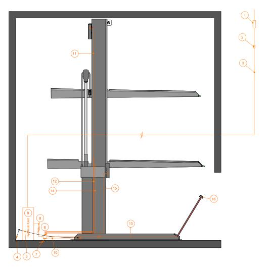
• During installation, it is required to appropriately connect electrical components with the wiring diagram supplied by the manufacturer in accordance with local regulations.
